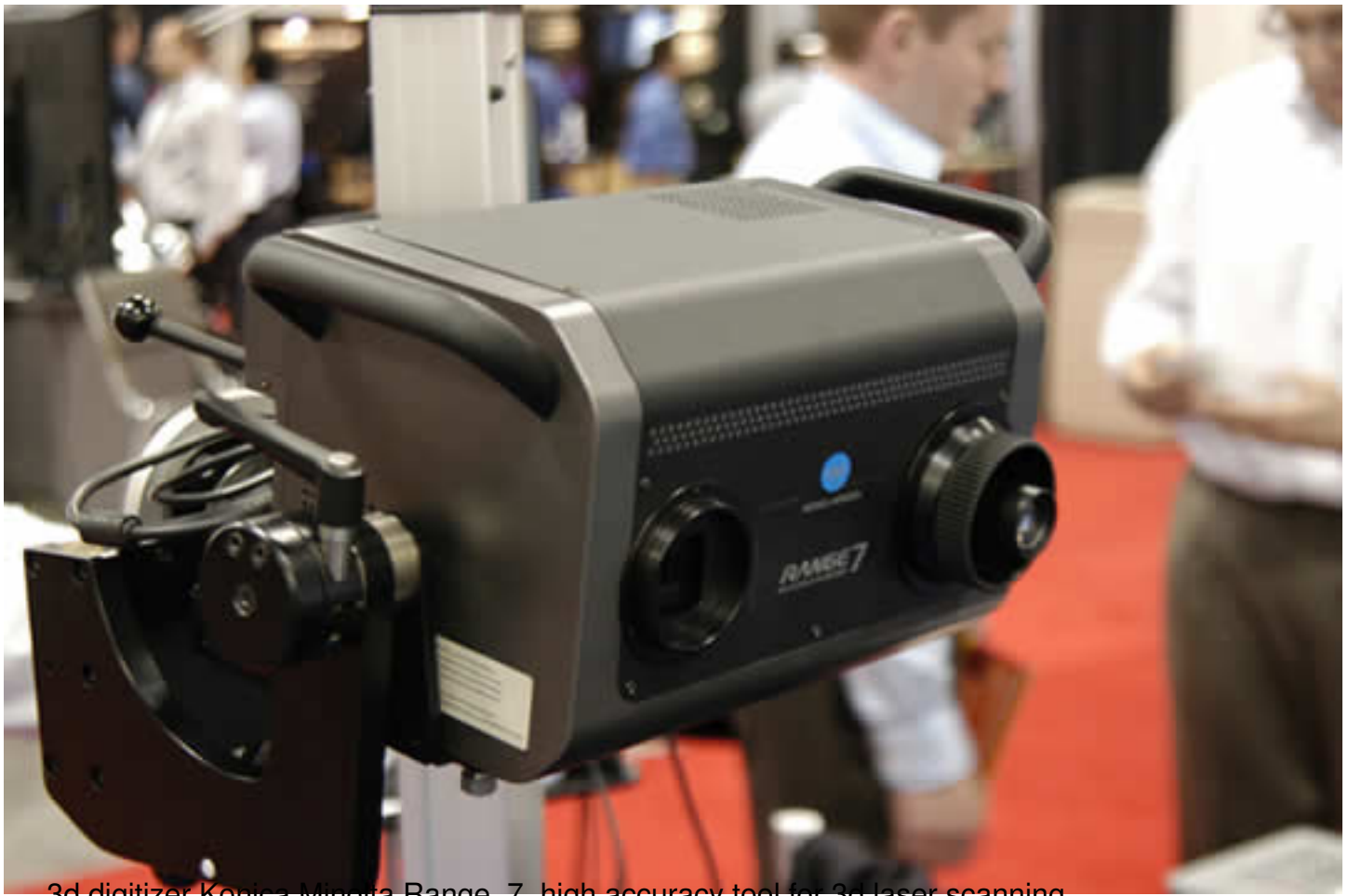
3d digitizer Konica Minolta Range 7, high accuracy tool for 3d laser scanning.
