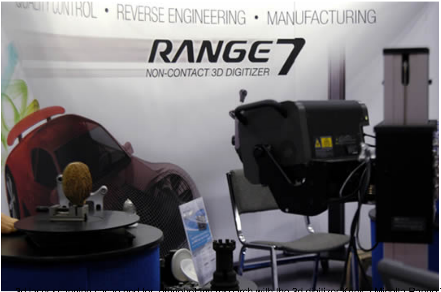
3d laser scanning cacao pod for ethnobotany research with the 3d digitizer Konica Minolta Range 7 a
